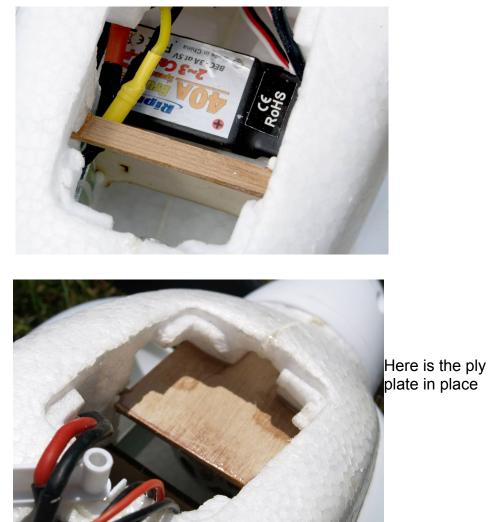
3 x 6 mm spruce cross-piece epoxied into the foam moulding
