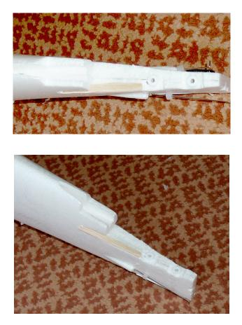
Too much glue had been splattered about on the aileron hinges and had to be trimmed off. It was underneath so was out of sight, but still not good. One positive was that the propellor was perfectly balanced and I mean perfectly. However the spinner was out of line with the fuselage so they have altered the thrust lines without changing the moulding. Or is this another misalignment? I won't know till I fly it.
